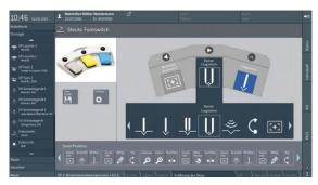
Fig. 3: The surgeon defines via touch screen or voice control which medical device is operated with the user interface
