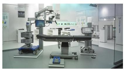
Fig. 2: Demonstrator for a user interface in the interoperable OR. The surgeon determines via a touchscreen or voice control which medical device should be controlled by the user interface.
